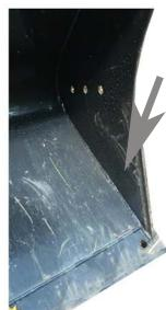
Measurement should be taken approximately 5" into bucket and 2" from bottom if no reinforcements on inside of bucket. Ignore any reinforcement on outside of bucket.
